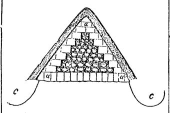
in which a a are sods, and c c the ditch all round the heap; potatoes and packing stuff, are the white and black space in the middle.
