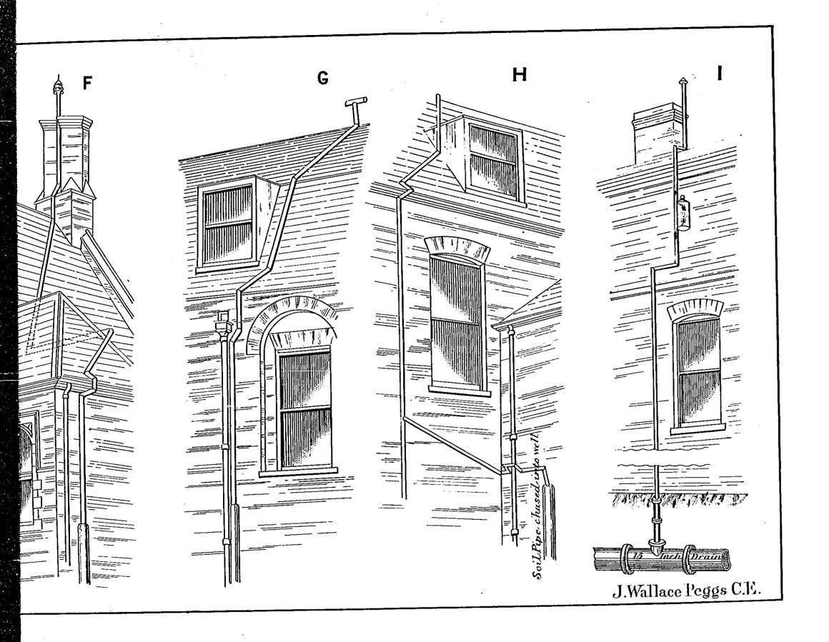
CASE D (Tottenham).—This illustrates another case of ventilating a 4-inch soil pipe by a 1-inch pipe carried up with numerous bends round the rain water pipe and stone coping.
