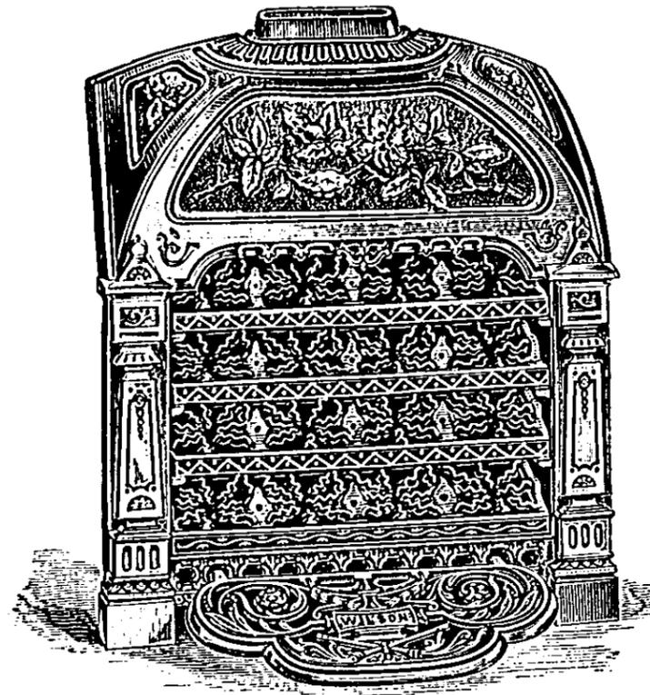
DESCRIPTION.—Metal Gratings of peculiar construction are placed between the bars in front and a Corrugated Fire-Brick Slab at the back of the fire. The iron bars are raised to a glowing heat by a series of Bunsen flames, and the heat reflected into the room by a Fire-Brick Slab. The fire can also be fitted on the hearth in front of the bars of a grate, on the tops of the bars, inside the grating, or on the Stands or Pedestals. The Burners are of an atmospheric type.
