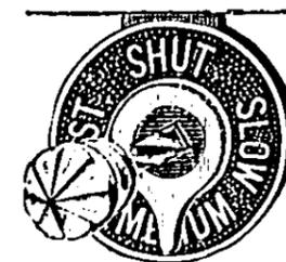
DESCRIPTION.—This shows on the front of the Range exactly at what draught the Range is working by indicating the position of the damper.
