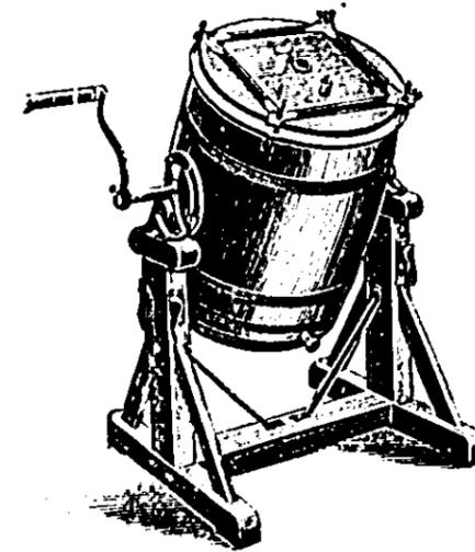
DESCRIPTION.—This Churn is in the form of a barrel, without heaters either fixed or movable, and revolves over end ways. The entire end of the Churn forms the lid; hence, there are no corners out of sight, and it is easy to keep it clean. Set into the lid is a glass window which admits of the contents inside the Churn being seen, thereby preventing overchurning.
