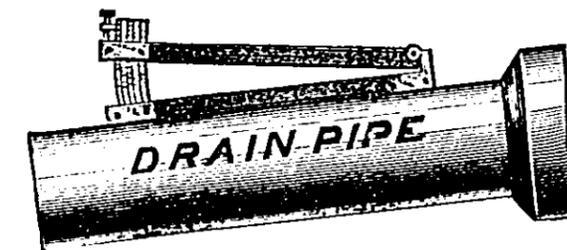
DESCRIPTION.—For the purpose of laying drain pipes at a given inclination. Generally used in conjunction with straight edge.
